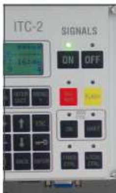
ITC-2: Compactly designed SWARCO ITC-2 with 16 signal-groups
